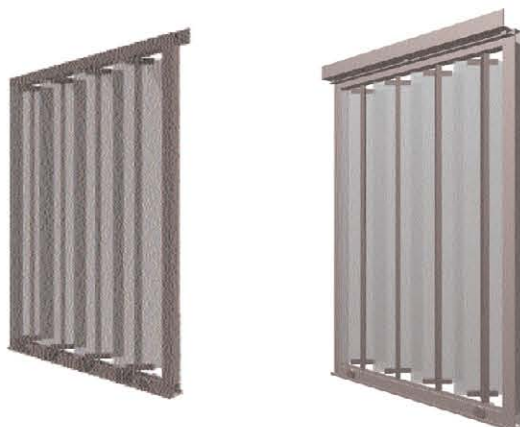
Fig.3: Shading device with grating hologram and absorber profile in Athens
