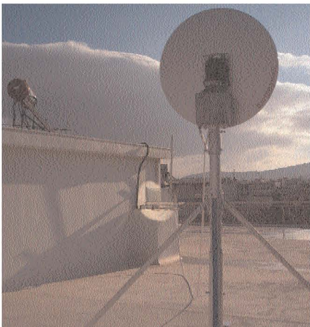
Fig.13: Sunlight redirection comprised in a heliostat and a white hologram for a Narrow Light Shaft in the building of STILVI Ltd.
